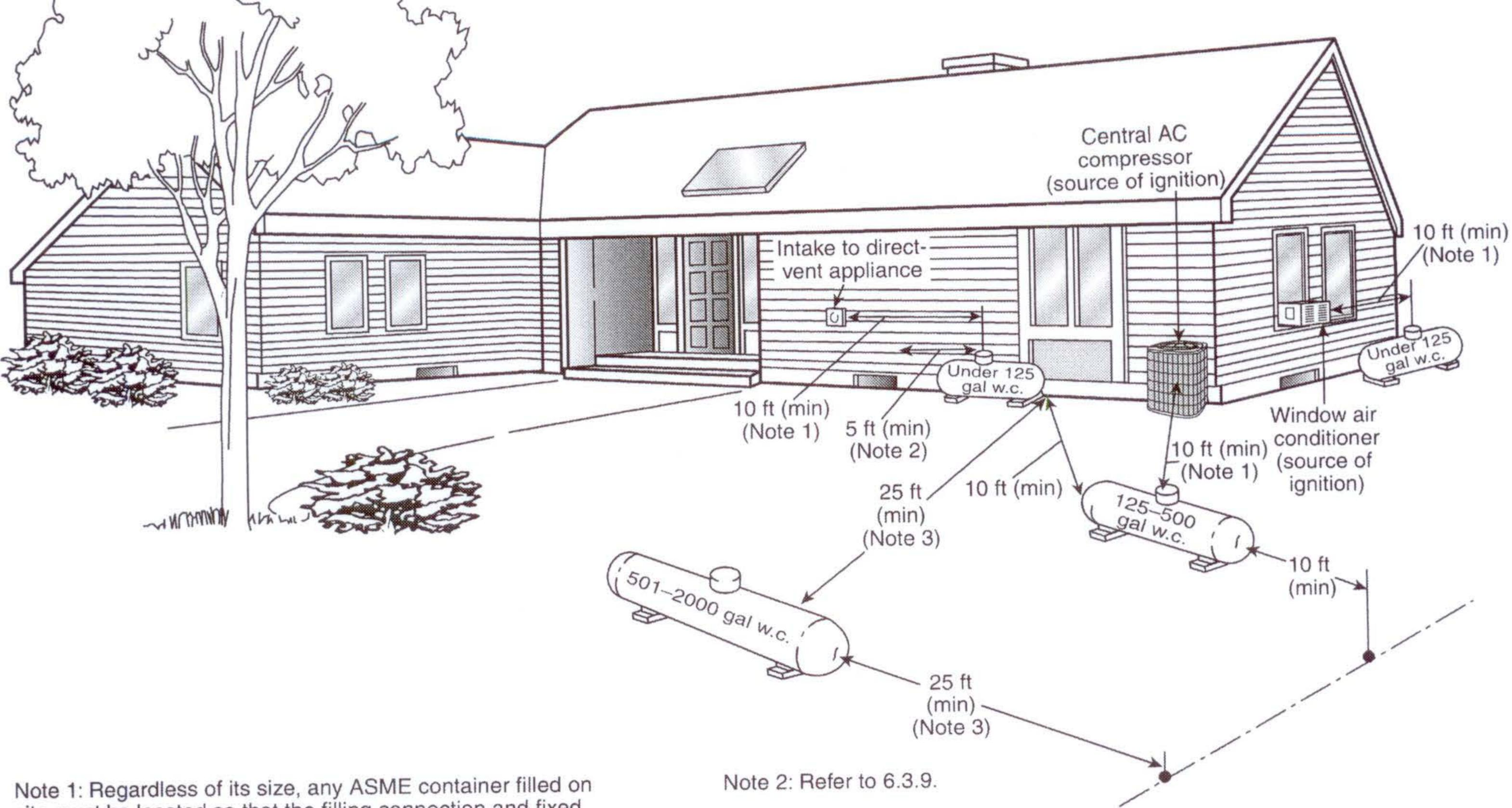
Note 1: Regardless of its size, any ASME container filled on site must be located so that the filling connection and fixed maximum liquid level gauge are at least 10 ft from any external source of ignition (e.g., open flame, window AC, compressor), intake to direct-vented gas appliance, or intake to a mechanical ventilation system. Refer to 6.3.10.
